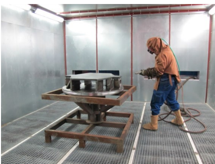
Manual blasting cabin 4.5x4.5 meters
