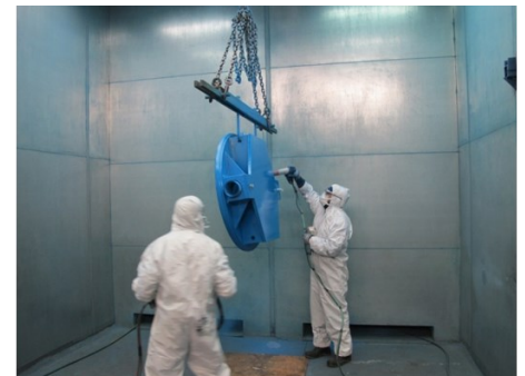
Manual powder coating, cabin 4x4 meters
