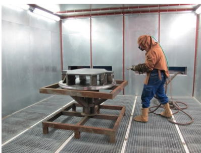
Manual blasting cabin 4.5x4.5 meters
